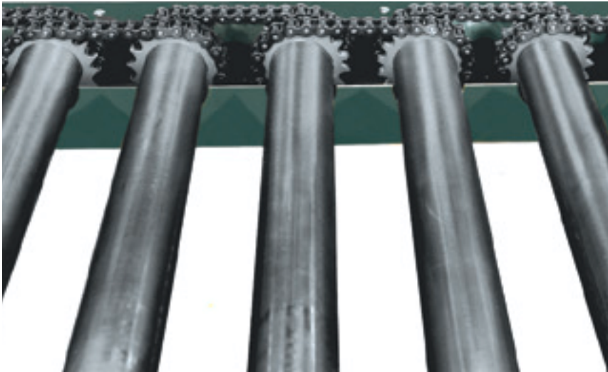
GUARD REMOVED TO ILLUSTRATE ROLL-TO-ROLL DRIVE CHAIN WARNING: Do not operate conveyor with Chain Guard removed.
