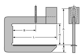
This model coil hook has a lower member length ("L" dimension) which equals the maximum coil width. The full length support feature increases the amount of surface area in contact with the coil, minimizing the potential for damage to the inner wraps of lighter gauge coil stock.
