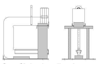
Because C-hooks are large and heavy, they can cause personal injury or property damage if they fall over. Each C-hook should be stored in an upright position on a stand specifically designed for its size, shape and weight.
