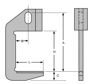
The model 610 C-hook is similar in construction to the model 624 (shown on following page). The lifting bail is turned 90° and burned from the same piece of plate as the hook, making it an integral part of the hook. The standard "H" dimension on the model 610 is 20". For variations in any dimension, please consult the factory with your application.
