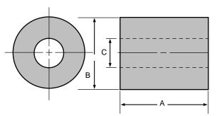
To ensure optimum C-hook performance, please provide the following important dimensional data (max./min.) for coil OD and ID and overall load length.
