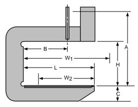
Designed for close stacking by shortening the distance from pick-up point (center of gravity) to the end of hook. Short lifting arm permits handling all coil widths within operating range (widest to narrowest) without the lifting arm extending beyond outer edge of coil. The reduced overall width of this style lifter can help decrease aisle space requirements, increasing storage capacity.
