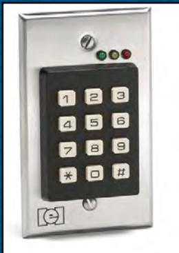
**(CE-2) Ten-Digit Key Pad...** operates electric strike or magnetic lock upon entry of four-digit pass code. Programmable up to 64 different codes. Available on hinged and sliding doors.
